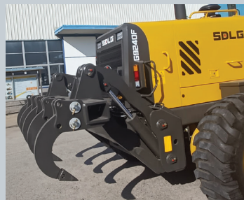
Rear Ripper The G9240F optional ripper is made to penetrate material fast and smooth thoroughly.
