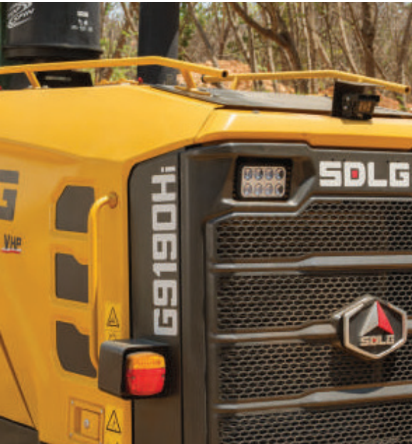
Handrails on engine hood for safe access to maintenance areas
