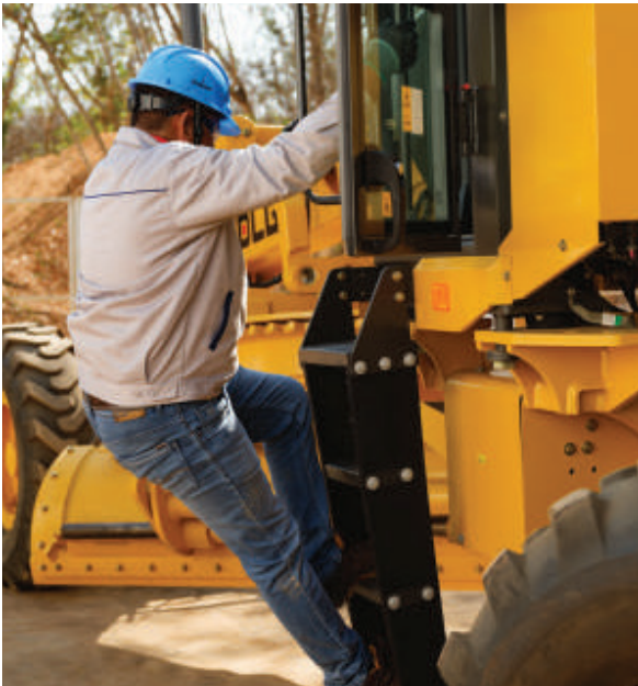
Seat belt, 3-point climbing access, and anti-slip perforated plates
