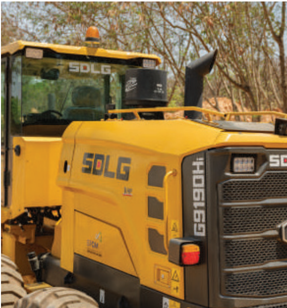
Extra Working lights, reverse horn, and rotating beacon for better visibility in low light conditions
