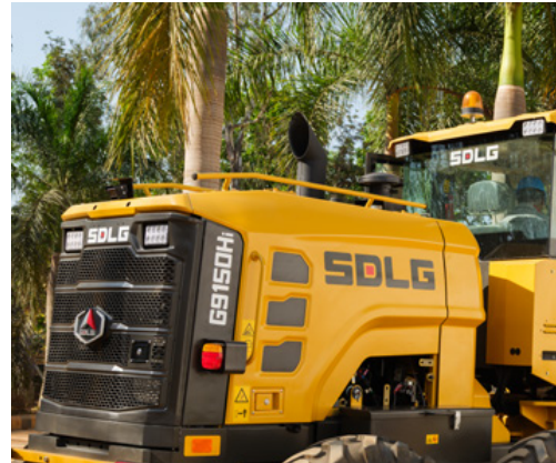
LED lights, reverse horn, and rotating beacon for visibility
