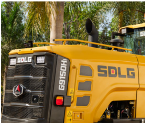
Handrails on engine hood for safe access to maintenance areas
