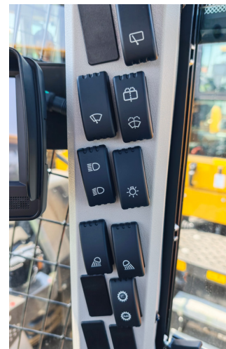
Pillar mounted function controls for ergonomic access
