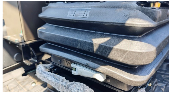
Weight-adjustable suspension seat for operator comfort.
