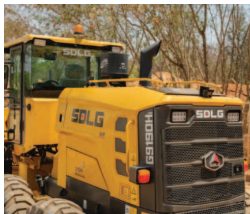
Extra Working lights, reverse horn, and rotating beacon for better visibility
