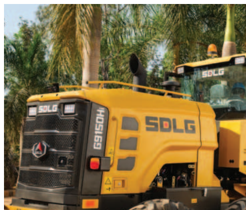
LED lights, reverse horn, and rotating beacon for visibility
